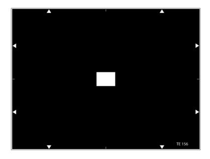
The test chart is designed to measure blooming and smearing effects of CCD cameras.
