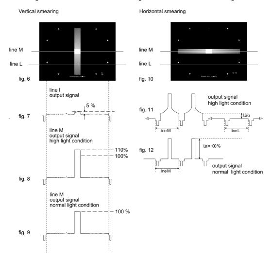
Note: In case there is no possibility to adjust the light density of the illuminator, ND filter shall be put in front of the camera. It shall be selected in such a way that the signal levels described above shall be attained. The density D of the ND filter, which attains the second signal level each, gives the result of the blooming and smearing ratios:  $10^D$
