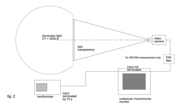
The output signal shall be measured by an oscilloscope.
