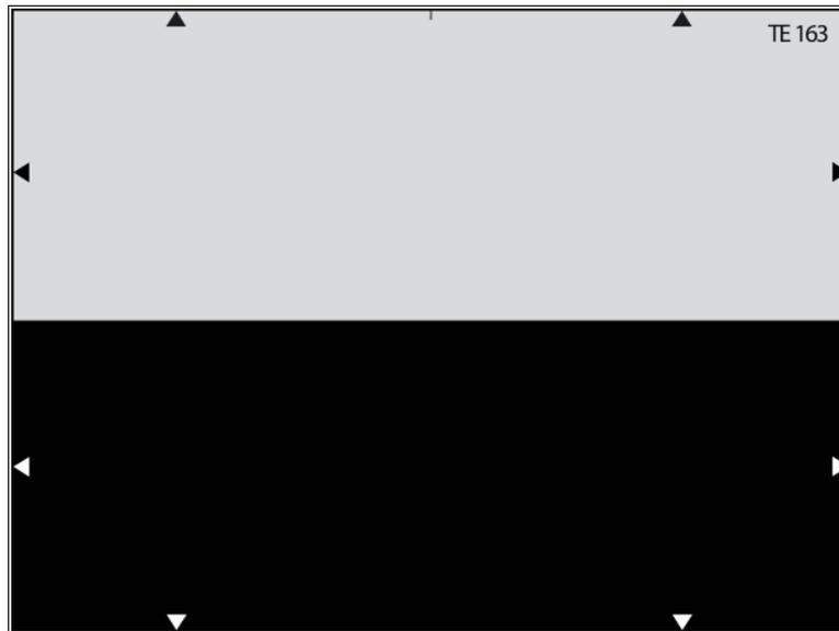
The test chart shows two picture halves in neutral gray and black. Gray has a remission (transmission) of 60% and black approx. 1.5%. The contrast range of both picture halves is 40:1 and thus corresponds to the contrast range which is recommended for television recording.
