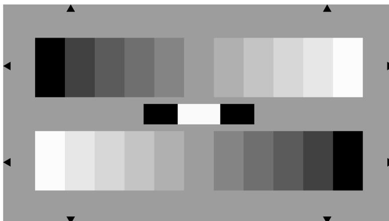
Two 11-graduated counter current gray scales are arranged on a gray background ( $D \approx 0.56$ ), the gray scale corresponds to the ITU recommendation BT.709.
