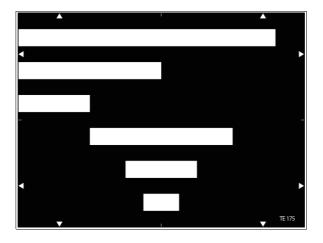
The TE175 is designed for measurement of the disturbance caused by the video level in black areas to the right of or below the areas. Horizontal white lines are positioned on a black background.
