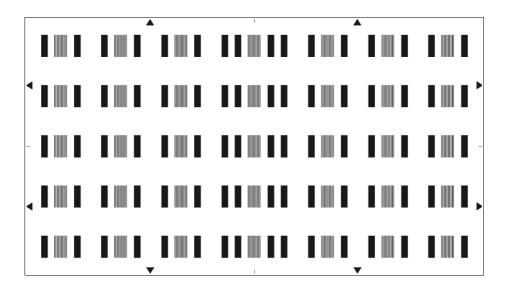
The test chart consists of alternating black and white bars with sharp transition (3-5 micrometers). The spatial variation of the density of these bars is a rectangular function of a cyclic ratio equal to 1. Two groups of bars with video frequencies of 0.5 and 5 MHz are distributed over the picture area whereby the 9 outer and middle positions each are essential for the measurements (the vertical, horizontal and diagonal axes, 10% within the extremities).
