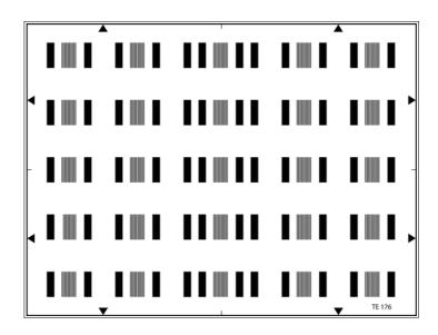
The test chart consists of alternating black and white bars with sharp transition (3-5 micrometers). The spatial variation of the density of these bars is a rectangular function of a cyclic ratio equal to 1. Two groups of bars with video frequencies of 0.5 and 5 MHz are distributed over the picture area whereby the 9 outer and middle positions each are essential for the measurements (the vertical, horizontal and diagonal axes, 10% within the extremities).
