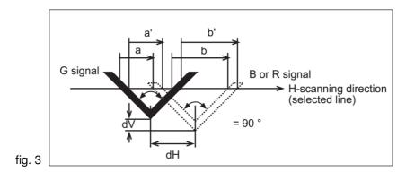
The segments a, a´-b, b´shall be considered as vectors whose origines are the crossing points of the selected line with "V" marks of the G-channel taken as reference is c for a, d for a´, e for b, and f for b´as exemlified in fig. 3. As to sign of a, a´, b and b´, the direction of the horizontal scanning is taken to be positive.
