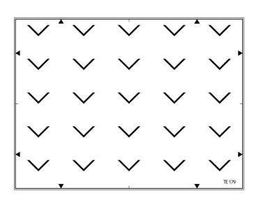
The TE179 is designed to measure fregistration of video cameras. The circuit arrangement of the measurement shall be as shown in fig. 2.
