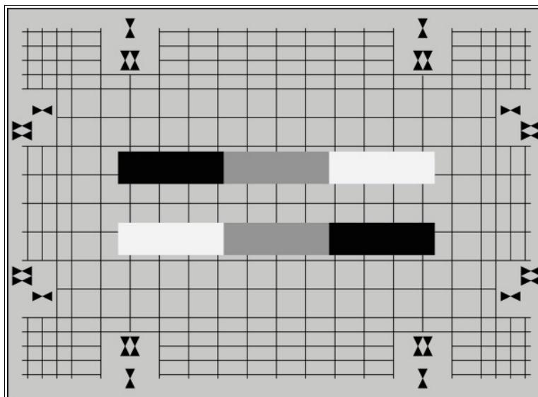
The IKEGAMI CPU-Chart is determined for setting up all IKEGAMI cameras which are switchable between 4:3 and 16:9 aspect ratio.
