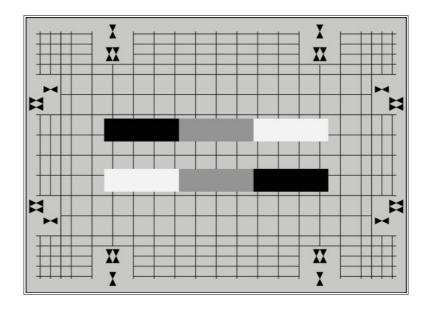
The IKEGAMI CPU-Chart is determined for setting up all IKEGAMI cameras which are switchable between 4:3 and 16:9 aspect ratio.
