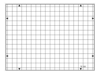
A grid structure of 14 horizontal and 19 vertical lines is arranged on a white background. The grid corresponds to a grid generated electronically by a test generator. The grid structure also corresponds to the ball structure of the T01 Geometry Test Chart.
