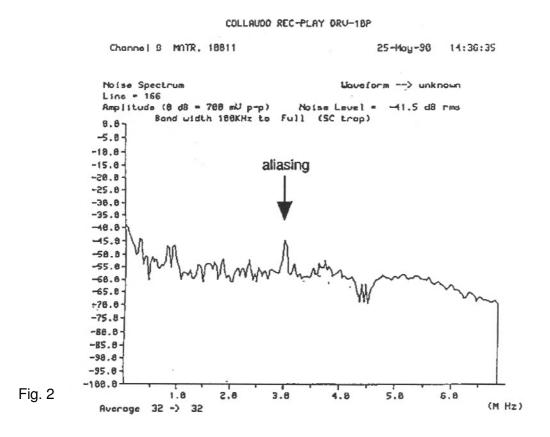
If the number of horizontal CCD pixels is known, it is possible to calculate the sampling frequency, which is easily located on the analysers screen:
