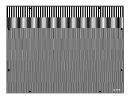
Aliasing effects are moiré distortions caused by interferences of two rasters. Independent of the type of camera aliasing effects can arise by interferences of motive rasters and the TV line structure e.g. the well known venetian blind effect or textile stripe patterns.
