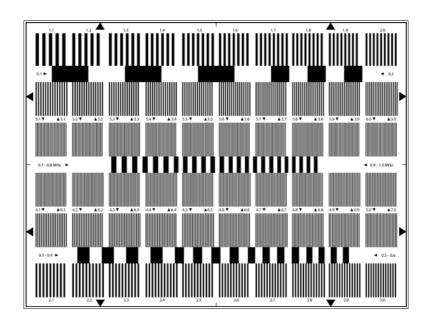
The test chart is designed for acute resolution measurement.
