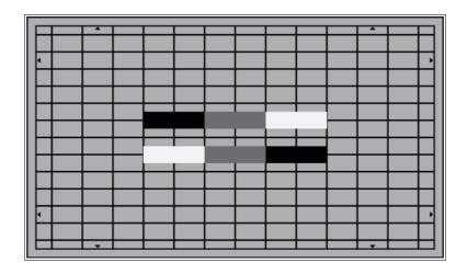
The SONY HDTV Setup Test Chart is designed for setting up all SONY cameras which are switchable between 4:3 and 16:9 aspect ratio.
