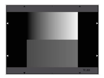
The TE203 is designed to check cameras for quantization errors. It consists of a high and low contrast saw tooth.
