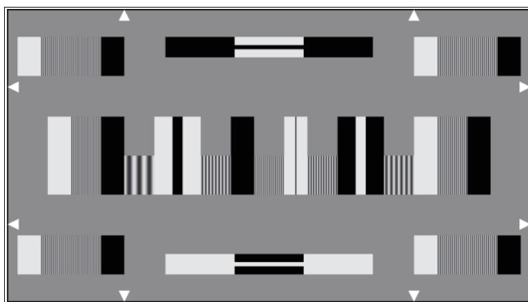
The TE204 is designed to measure resolution of cameras.
