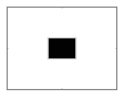
The TE206 is used to measure flare of camera systems.
