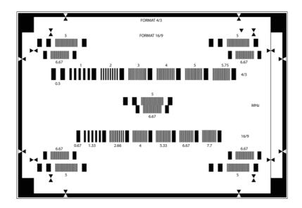
The TE207 is designed to measure resolution.
