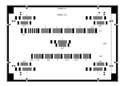
The TE207 is designed to measure resolution.
