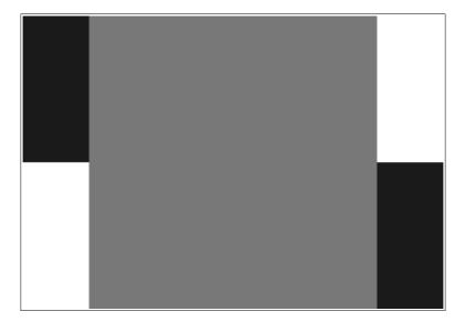
The test chart shows in its center a field of neutral gray with 18% reflectance and at its sides 2 small fields each with white of 90% and black of 3% reflectance.
