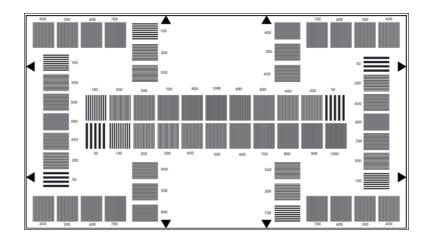
The TE224 is designed to measure and describe the frequency response of an electronic HDTV camera.
