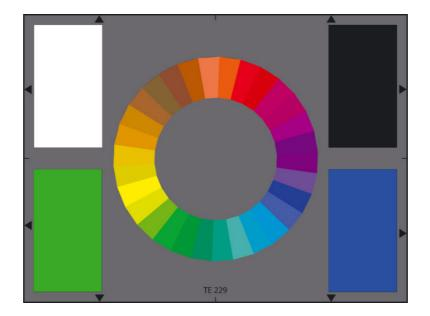
The TE229 is designed to check colors of a camera.
