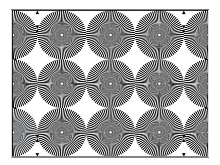
The TE237 serves for checking resolution over the whole picture area.
