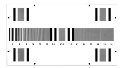
The TE239 is designed for checking the frequency response of modulation depth and the uniformity of modulation depth of HDTV cameras.
