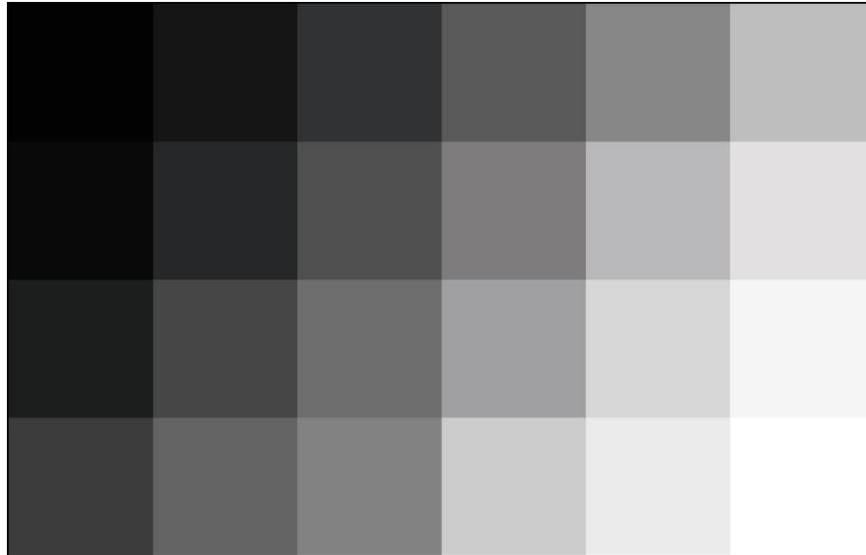
The TE240 D is designed to determine the dynamic range and the scanner opto electronic conversion function (OECF). The OECF describes how the scanner transforms luminance values of the object into digital code values in the digital image. The OECF is typically measured from a gray scale.
