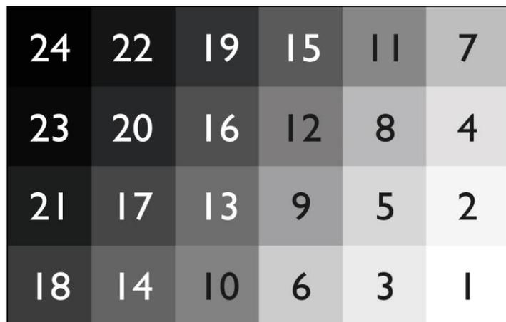
In order to measure a scanner, the contrast of the chart should exceed the dynamic range of the camera under test. The TE240 D is therefore available in the contrast ranges 10.000:1 and 1.000.000:1.
