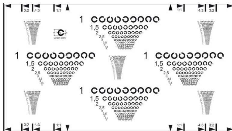
The TE245 is designed to make a visual resolution analysis of digital cameras.
