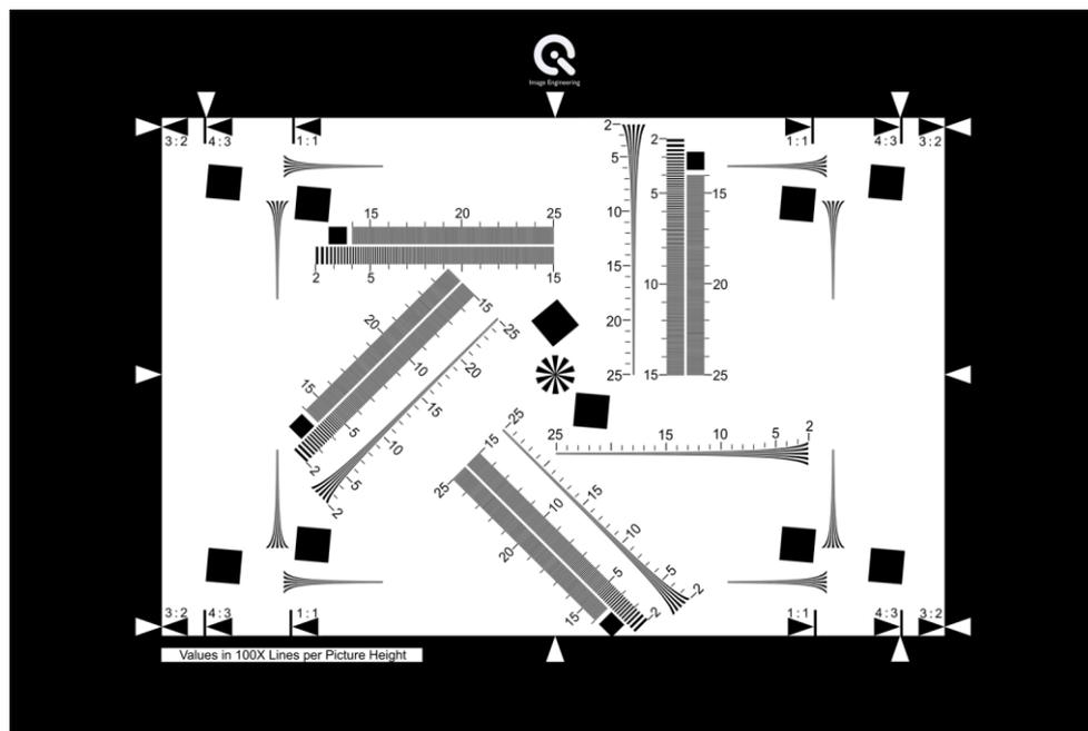
The TE252 is designed to measure resolution of digital cameras.
