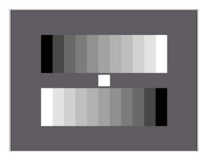
Two 11-graduated counter current gray scales are arranged on a gray background (D $\approx$ 0.65), the gray scales being graduated linear. Related to the densities of the gray scales: gamma = 1. The contrast range of the gray scales is 40:1.
