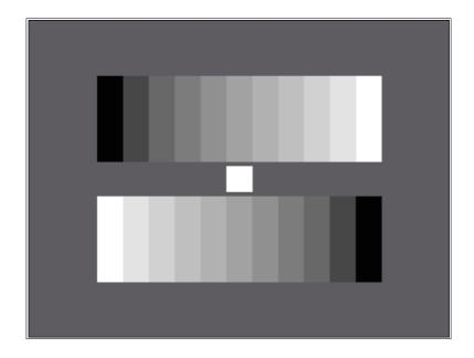
Two 11-graduated counter current gray scales are arranged on a gray background ( $D\approx0.65$ ), the gray scales being graduated linear. Related to the densities of the gray scales: gamma = 1. The contrast range of the gray scales is 40:1.
