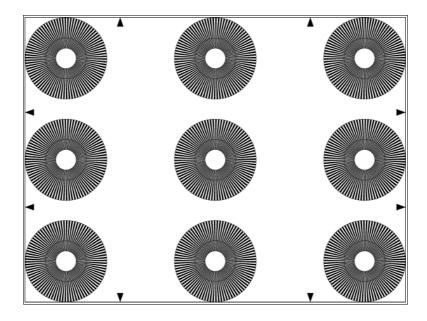
The TE94 consists of 9 sector stars of 90 (black and white) sectors each. The diameter of the unresolved middle and the outer diameter are marked by circles. A further marking circle is positioned within each sector star. The circles are marking the following resolutions:
