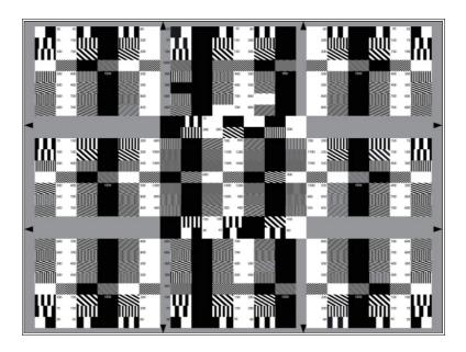
The TE96 is designed to measure aperture dependent on resolution in the field.
