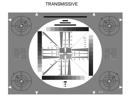
The TE97 corresponds to the 4:3 part of the HDTV test chart TE117. It is designed for measuring and quick (most visual) appraisal of transmission characteristics of high resolution non-broadcast cameras.
