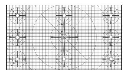
The TE98 is designed to do a geometrical camera alignment.
