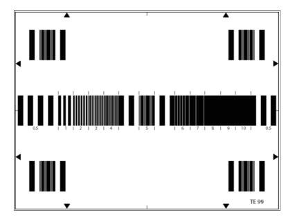
A line raster is arranged in the center of the test chart which produces frequencies of 0.5 to 10 MHz in the output of the TV camera. 0.5 MHz line pairs are also arranged at the center of the line raster immediately adjacent to the 5 MHz line pairs. Bar rasters are located in the corners of the test charts and produce frequencies of 0.5 and 5 MHz.
