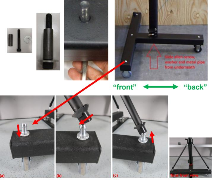
The three stabilization arms must be adjusted on the metal holders. Screw the holders to the down position (a), push the arm onto the holder (b), and screw the holder up (c) until the construction is stable. Steps (a) to (c) should be done by hand and not with a tool to avoid an over-tight adjustment.
