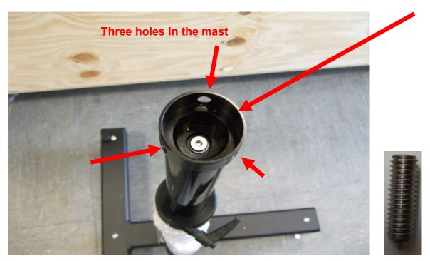
There are three holes with threads on the mast's upper side. These threads are used to anchor the H-shaped height adjustment to the mast.
