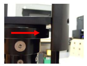
When you fix the H-shaped height adjustment to the mast, please loosen the screw connecting the T-base with the mast and align all parts. Then tighten the big screw to the T-base again permanently.
