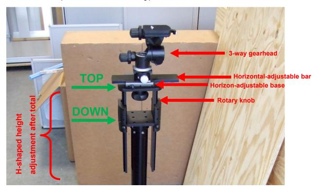
The base of the horizontal-adjustment bar has a trapezoidal bar. You can fix the 3-way gearhead on the plate of the horizontal-adjustment bar and slide the plate into the side of the horizontal-adjustment base.
