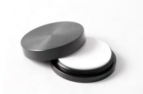
The white reference RESTAN based on PTFE (Polytetrafluoroethylene) diffusely reflects more than 98% of light in the area between 300nm and 1700nm. This means the reflection level is higher and more uniform especially at longer wavelength than the reflectance of barium sulfate (BaSO<sub>4</sub>).
