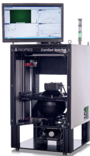
Production line integration for camera control testing within the CamTest Spectral module from Trioptics GmbH
