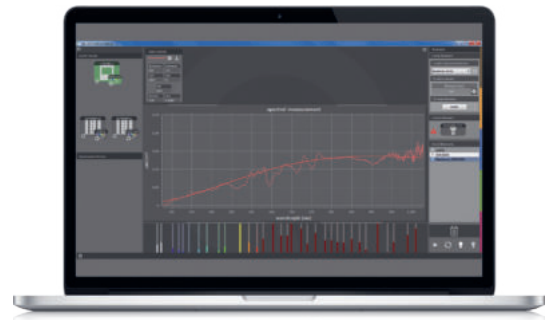
iQ-LED software main screen with 32 spectral channels
