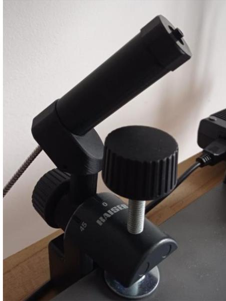
Set up the device in an upright (0°) position, as shown in the image above, so it 'looks' into the illuminated scene.
