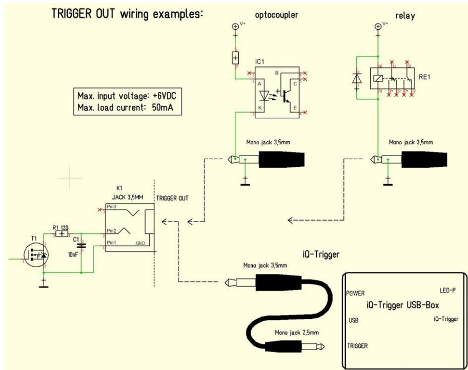
The default duration value for the trigger output is 500 ms. This value can be modified with the iQ-LED API. A signal is sent out to the trigger output while changing the illuminants or the intensity of LED channels. It can be used to synchronize your test setup. For example, with an iQ-Trigger. (See 2.1 optional equipment)
