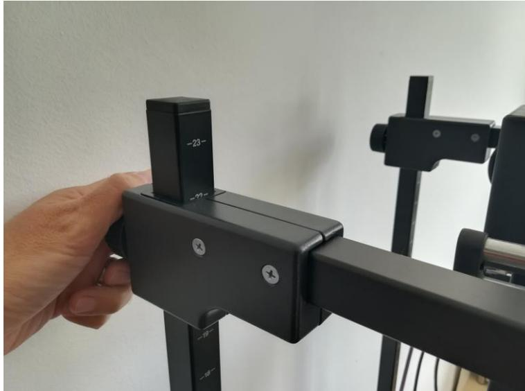
Bring the lamps into a 45° position and lift them to the same height of about 40cm. You can also use the lower corner of the lamp as a reference point for determining the height.
