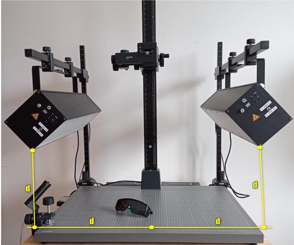
Once the positioning is correct, begin measuring the uniformity of illumination on your test chart and adjust the position of your lamp units to best suit your test setup. We recommend using an exposure meter (see 2.1 optional equipment) to check the uniformity of the light. Measure all four corners and the center of the chart. The values shouldn't deviate 10% from each other.
