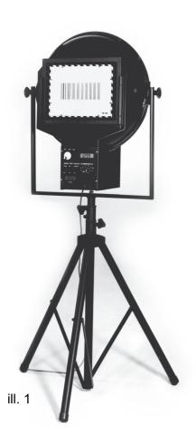
The spherical transparency illuminator LE6-50 is designed for illuminating test transparencies of all kinds that are used for testing and evaluating visual recording equipment, mainly electronic cameras. The transparency format is 360x280x4mm. When using other formats an adapter is necessary.
