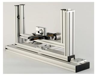
possible to move just yaw or pitch or to move both of them together. The frequency and angle can be set for each direction individually. A well-defined movement in yaw and pitch axis is produced and logged. The type of movement can be as simple as a sine wave or an individual setting e.g. to simulate a real handshake.
