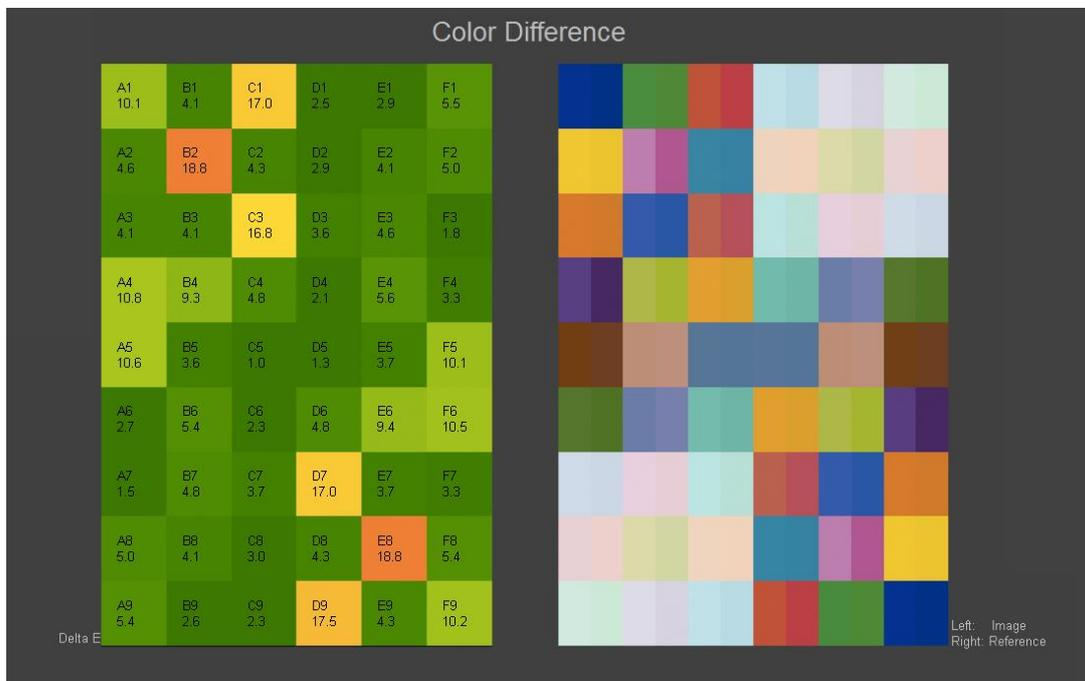
On the left side the numeric results for each patch are shown and the amount of the color difference is visualized by colors - from dark green ( $\Delta E = 0$ ) to dark red ( $\Delta E = \text{maximum value defined in the specification}$ ). On the right side a visual comparison of the color patches are shown (left: image, right
