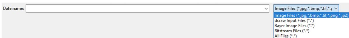
By changing the file type iQ-Analyzer is triggered to check and execute the settings within the RAW module. Delete selected files with the “-“ button and clear the list with the “C” button.
