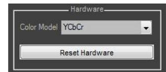
Press the „Reset Hardware“ button if you have connected or detached a hardware device. The search for the available devices is performed without the necessity to restart the iQ-Analyzer.
