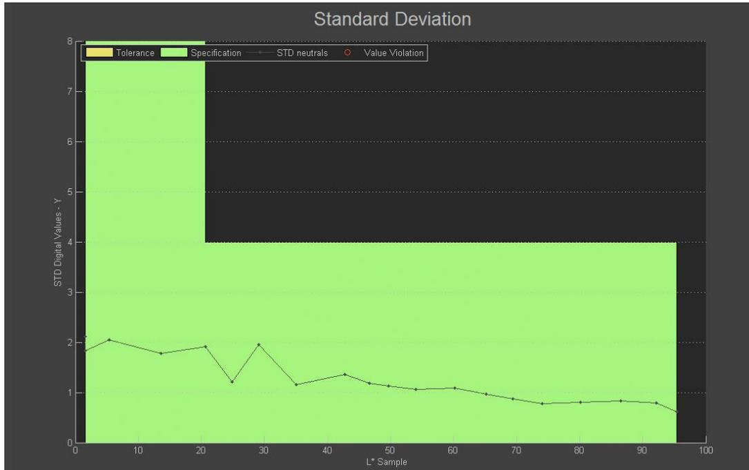
The tolerance range, that is defined in the specifications, is displayed in green. Values that are outside the tolerance range are outlined in red „Value Violation“.
