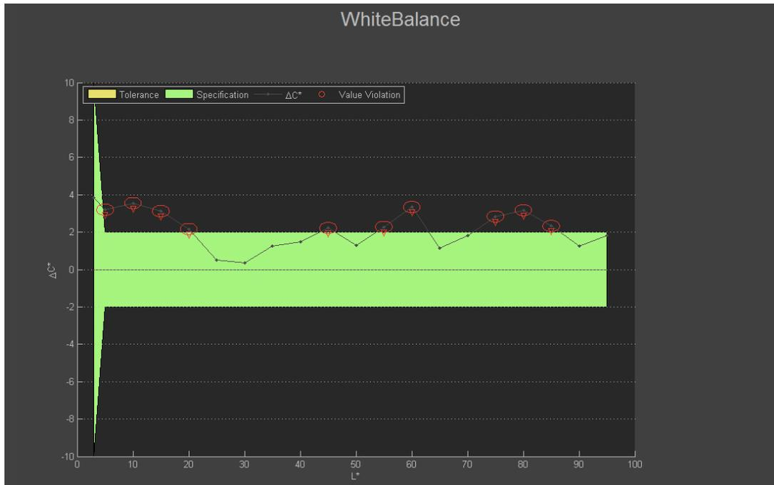
At best  $\Delta C^*$  is 0 (no color cast). The tolerance range, that is defined in the specifications, is displayed in green. Values that are outside the tolerance range are outlined in red „Value Violation“.
