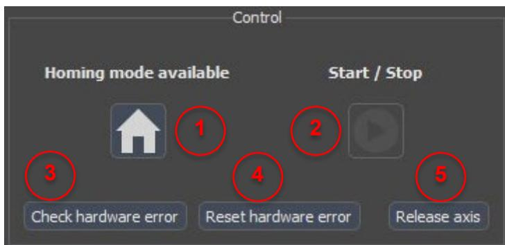
The control panel is used for homing functionality, start/stop of movement and error handling.
