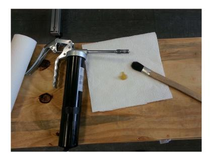
Lubricate the guide rods and the lubricating felts with <u>"Klüber Isoflex Topas NCA 52"</u>
