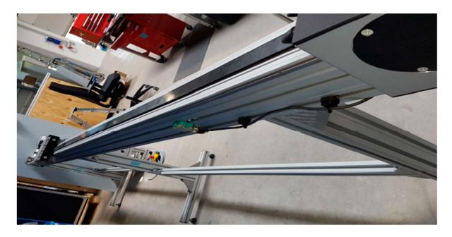
Secure the bench to the feet with hammer screws.
