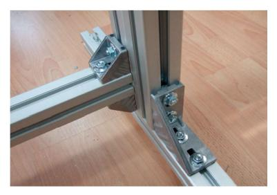
First, put the aluminum bars in position THEN slide in the screw. Pull the screw to the very front position and tighten it by hand. Make sure the hammer slips into the correct position. When the screw is secured, you can use the wrench to tighten it.
