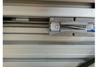
The lubrication should be implemented annually with the following grease: "Klüber Isoflex Topas NCA 52".
