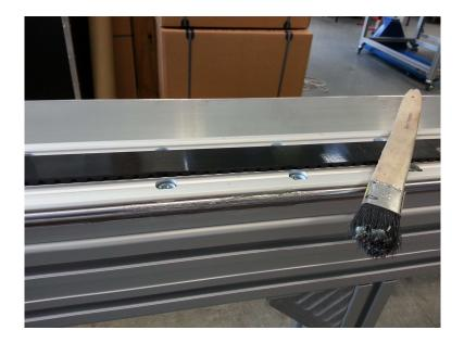
Lubricate the guide rods and the lubricating felts with <u>"Klüber Isoflex Topas NCA 52" (see the Fig 1)</u>
