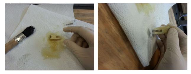
The lubrication should be implemented annually with the following grease: "Klüber Isoflex Topas NCA 52".
