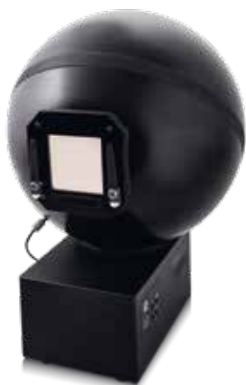
A modified CAL1 for size D35 transparent test charts
