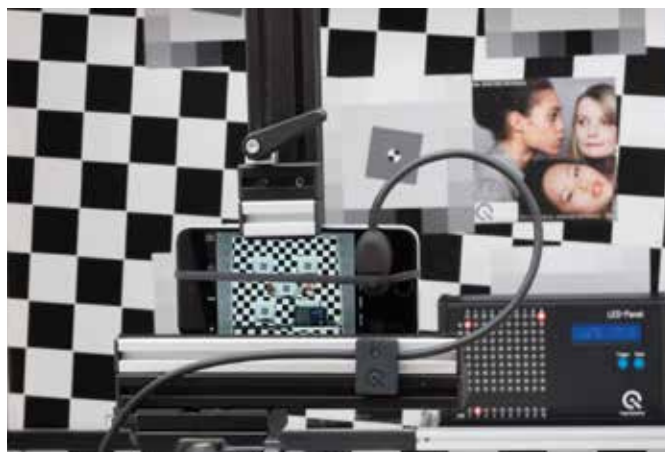
An example of a timing measurement test
