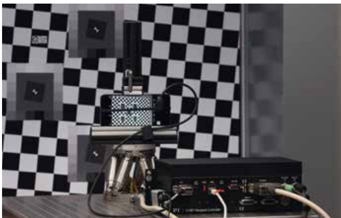
Camera stabilization measurement with the iQ-AF Box
