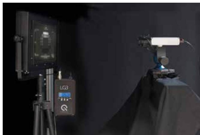
An example of a security camera test with the LG3
