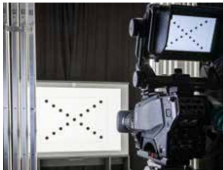
Testing for camera flare
