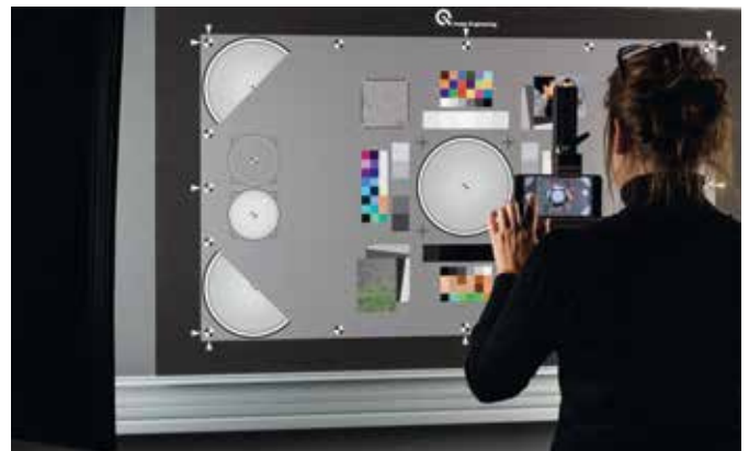
VCX testing with the TE42 multipurpose chart
