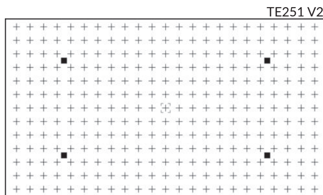
Geometry grid to measure lens distortion
