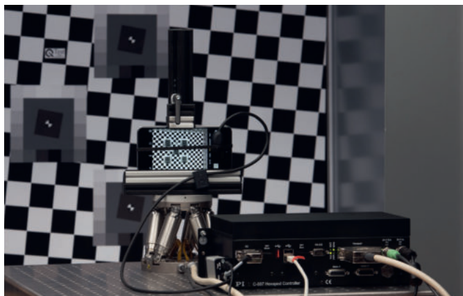
Camera stabilization measurement with the iQ-AF Box
