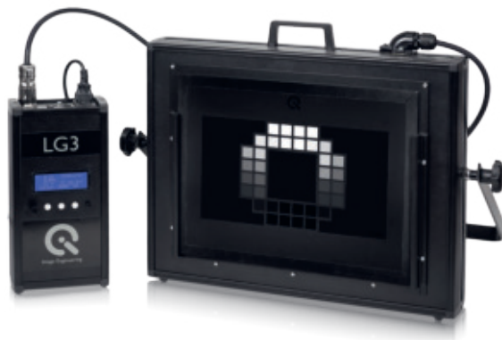
LG3 with OECF test chart TE269C
